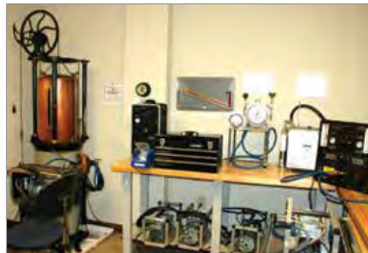
Calibration being performed with Wet Test Meter
