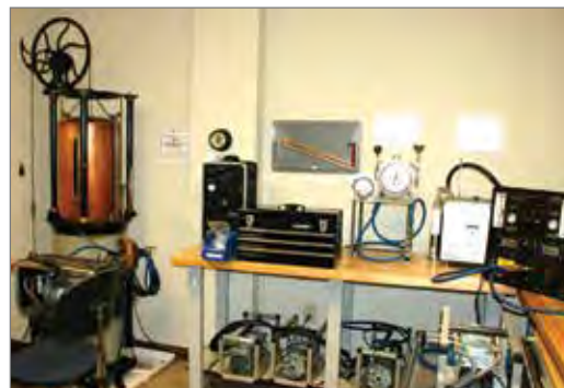
Calibration being performed with wet test meter
